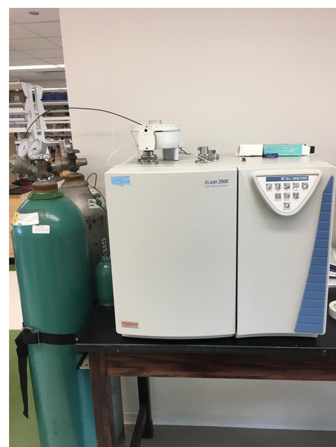
Image 3: Flash 2000 Organic Elemental Analyzer for protein content analysis.
